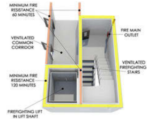
Fig 9.2.1: Components of a firefighting shaft residential buildings only
