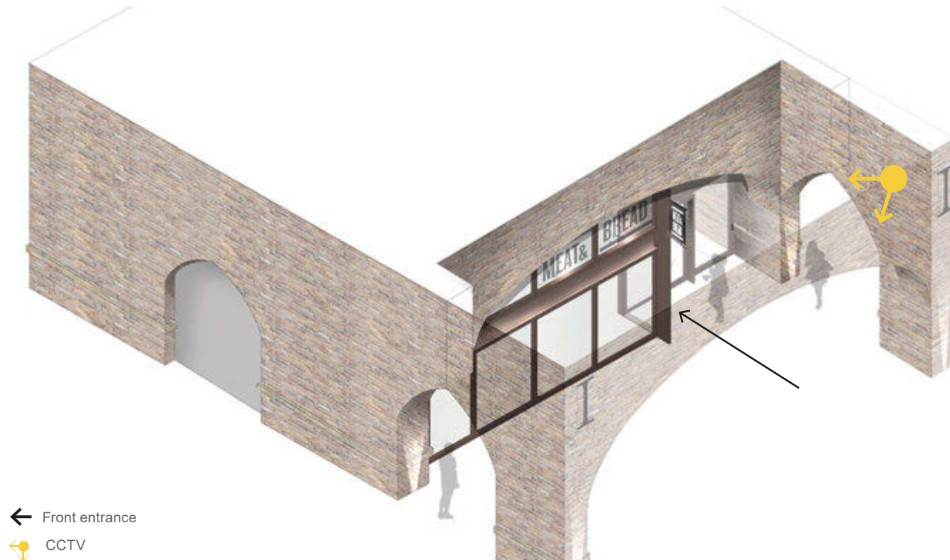
Fig 8.2.4: Axonometric of a typical A1 cafe shopfront, with a recessed doorway, set back from the viaduct frontage
